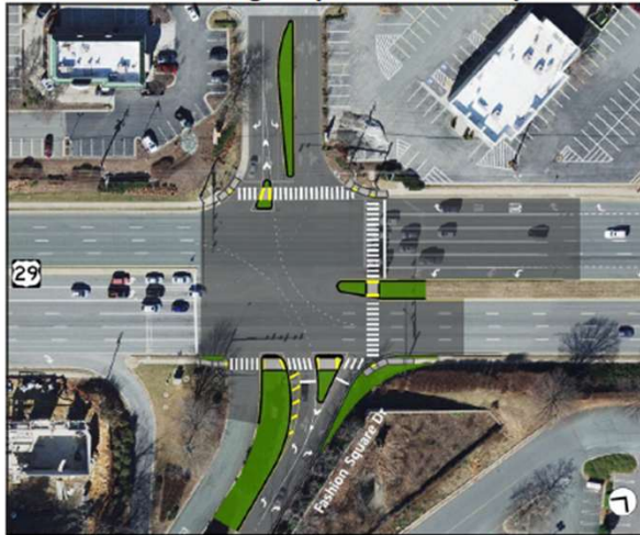
Pedestrian Crossing Improvements (Thru-Cut)
